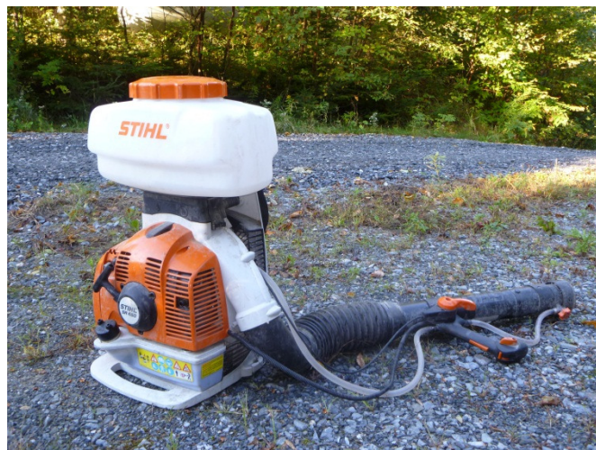
Figure 9. A mist blower backpack sprayer. Photo courtesy of Courtney Haynes.
