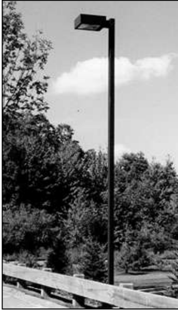
Although not very attractive, this "shoebox" fixture sheds light only downward.
