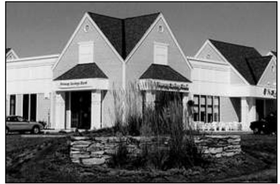
Modulated building forms and variation of roofline reduce the scale, while similar materials create cohesiveness.
